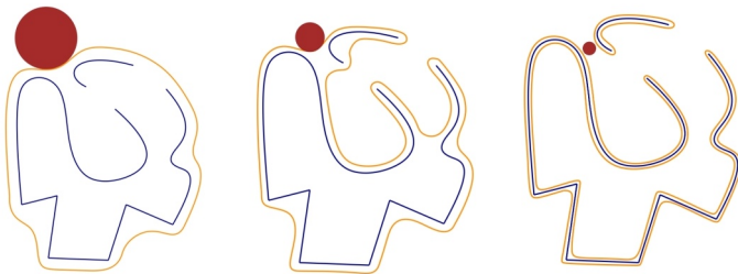
Figure: Alpha Wrapping in 2D with Offset and different Alpha parameters
