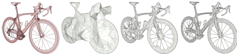
Figure: Different LOD of the Alpha Wrapping of a bike[5]
